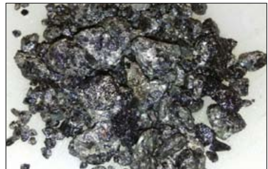
Photo 1: RC Chips containing up to 20% massive sulphides pyrite and chalcopyrite. FRRC021, 21-22m.
