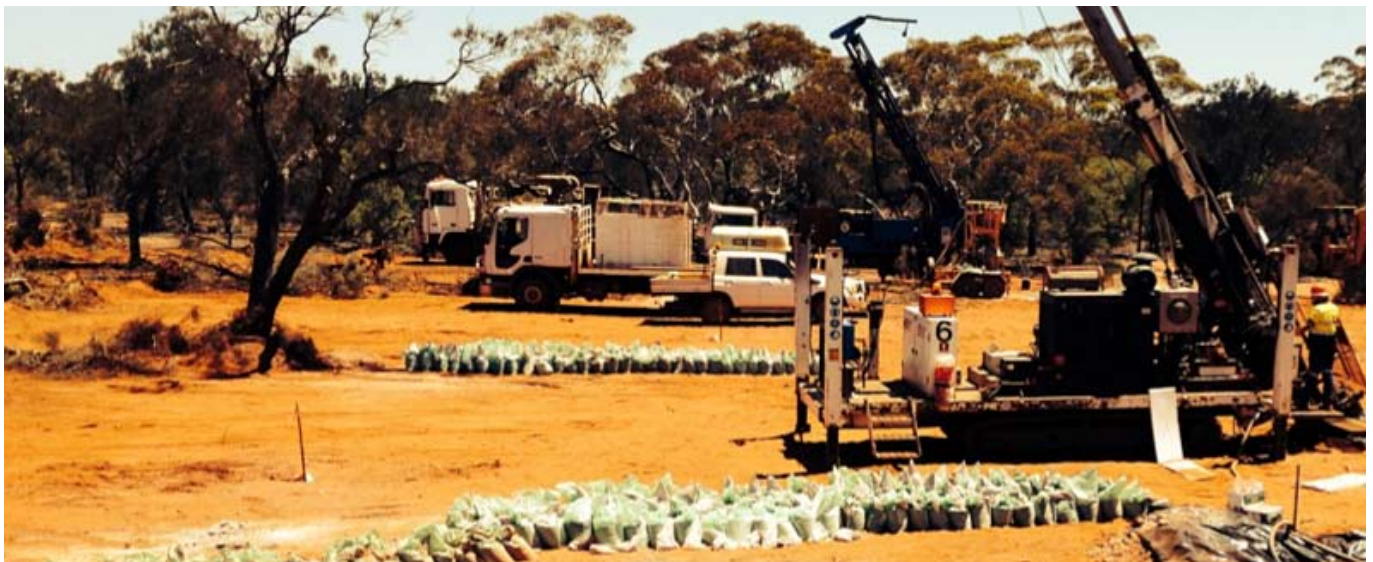
Figure 2. RC and Diamond Drilling in progress at Mammoth target
