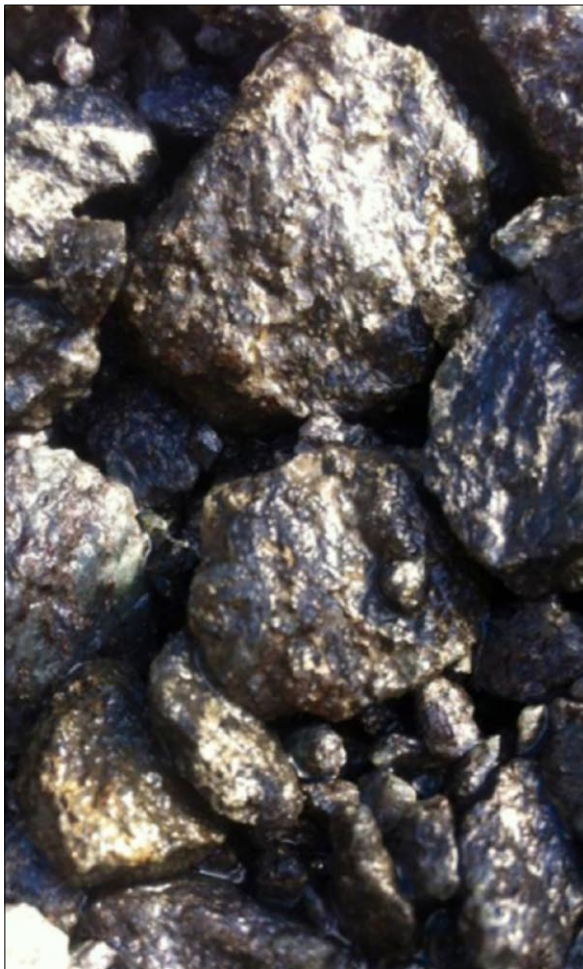
Figure 1. A17 Visual Fe Zn Cu sulphides in latest drilling program. Chips are from FRRC075 at 61-62 metres downhole. Chips are 20mm to 3mm in size.
