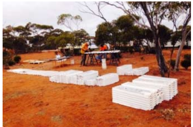
Image 2: Geologist and field personal logging NQ2 core at the Fraser Range Project
