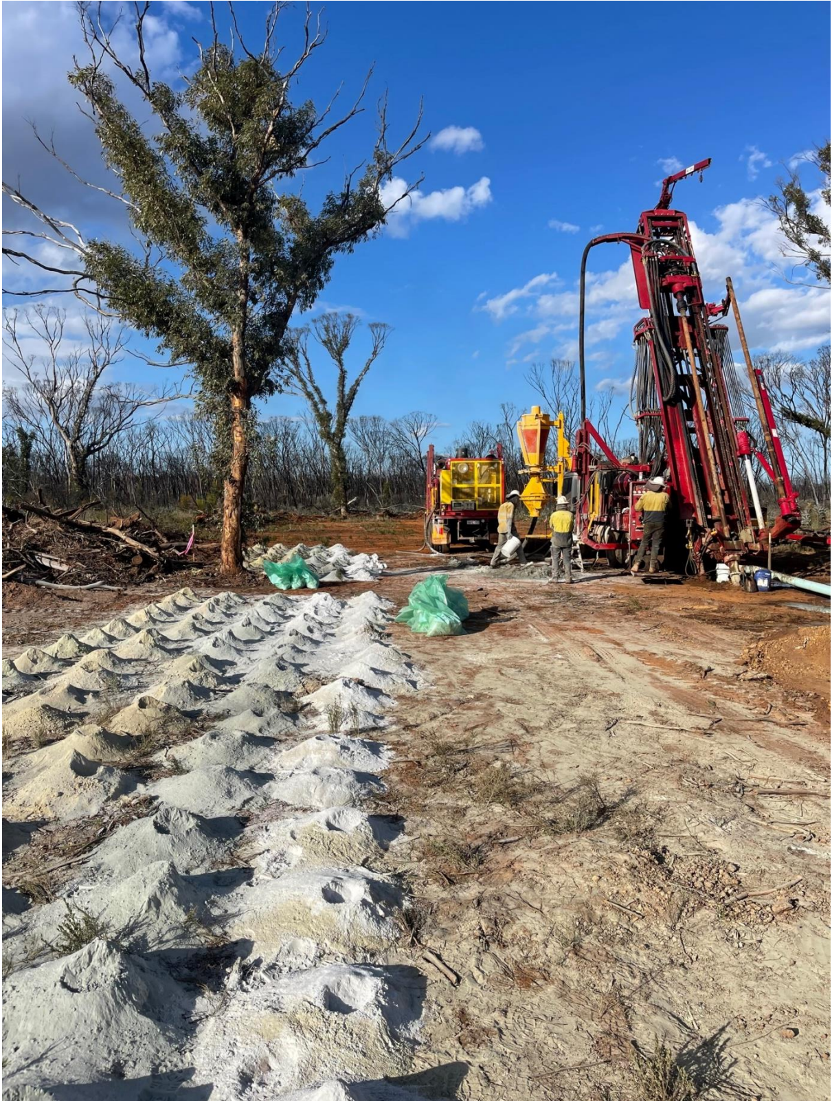
Figure 2: Extensional RC Drilling at Kat Gap
