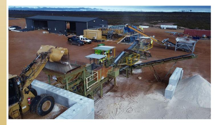
Figure 1 – Hopper at Crushing Circuit being loaded at Kat Gap.
