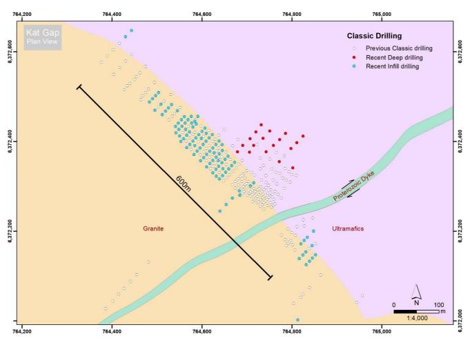
Figure 3: Infill and deep RC drilling at Kat Gap
