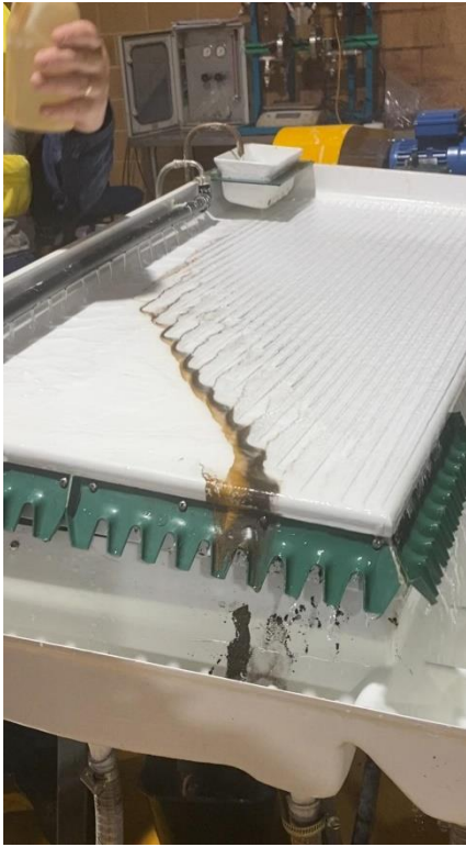
Figure 1: Gold from Kat Gap ore across Met shaker table Figure 2: Kat Gap Gold from Gekko spinner concentrate
