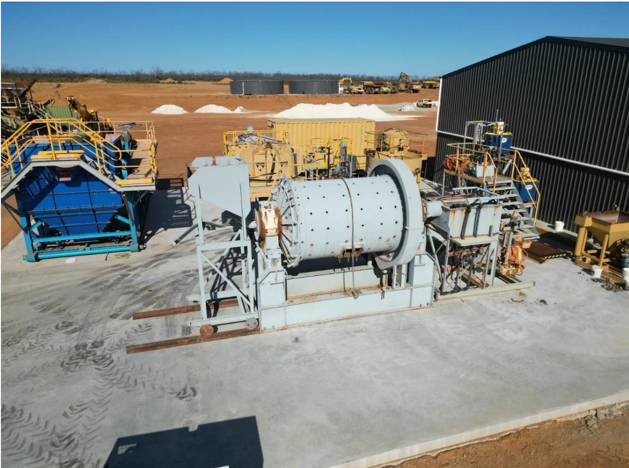
**Figure 10: Picture showing Ball Mill, Trommel and water tanks.**
