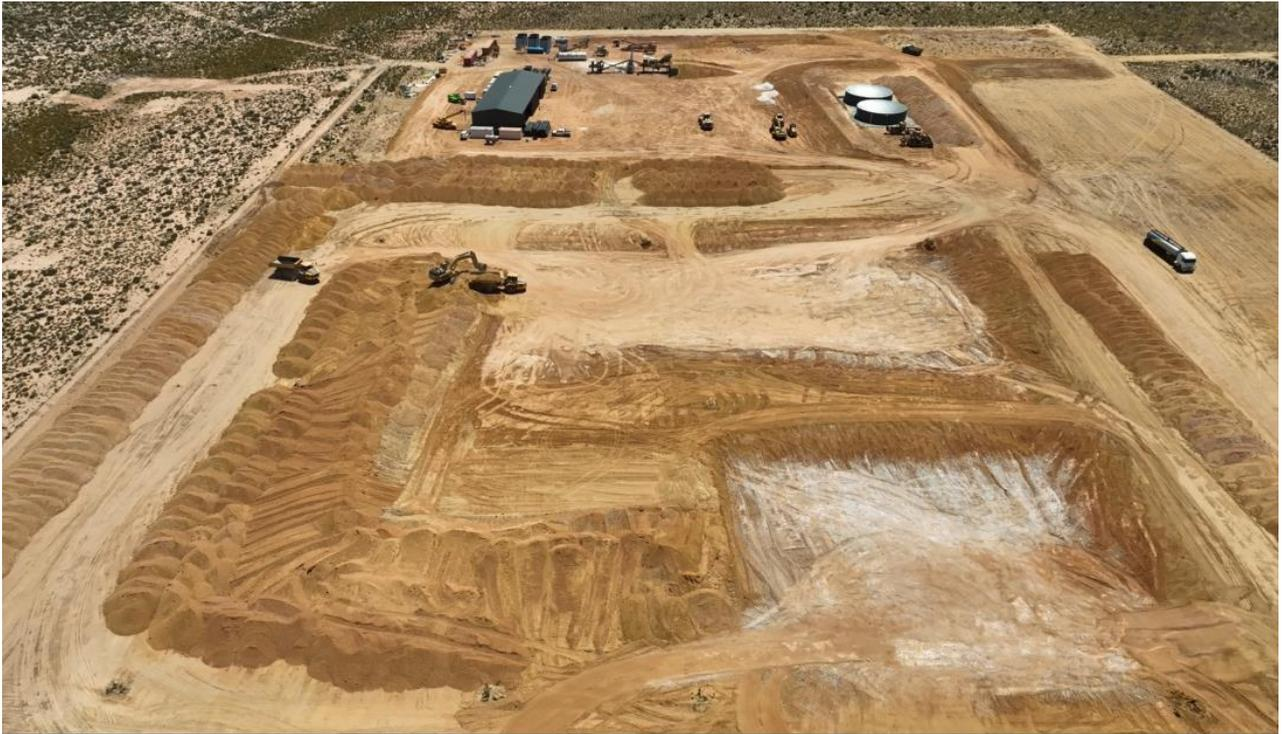
**Figure 2: Aerial photo of Kat Gap Processing Facility showing TSF progress.**
