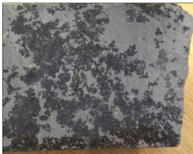
Figure 1: Core hole FRDH001. Massive -blebby Sulphides in FRDH001 at 41.7m downhole. Core is 50mm wide. The pale grey is pyrrhotite and the yellow is pentlandite and chalcopyrite
